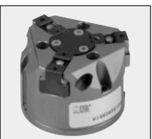
Highly-accurate sturdy grippers guaranteed for 1,500,000 cycles at maximum load without requiring maintenance. Top quality materials and accurate working. Highly resistant hardened aluminium alloy body. Moving parts made of tempered steel. Double action with internal or external clamping. Magnets for position sensors, except for size 50 which can mount induction magnets.
